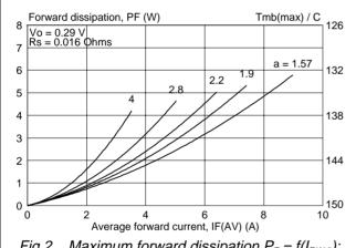
Fig.2. Maximum forward dissipation  $P_F = f(I_{F(AV)});$  square current waveform where  $I_{F(AV)} = I_{F(RMS)} \times \sqrt{D}.$
